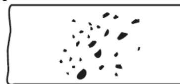
(a) Random Rounded Indications Typical concentration and size permitted in any 150 mm length of weld.
